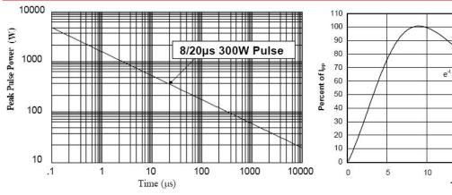
Figure 1. Peak Pulse Power Vs Pulse Time ( $\mu$ s)
